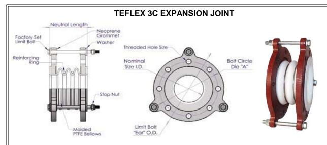
The Teflex expansion joints are composed of unreinforced PTFE and come standard with iron 150# drill flanges. Stainless flanges are available as an option. They are available in 2, 3, or 5 convolutions of varying movements. The 3-convolution joint shown here is sometimes referred to as a "bellows".
