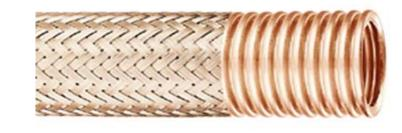
BB1 & BB2 are corrugated bronze hoses with a single and double bronze braid. It has a high pressure capacity at high temperatures. It is resistant to bursting, cracking, and crushing even under accidental exposure to flame, while being quite flexible and resistant to vibration. -50F to 450F.
