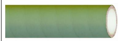
The Model RH1 is a heavier weight rubber material handling hose designed for a variety of slurries and dry highly abrasive materials throughout industry. It uses an FDA Grade, thick, smooth bore natural rubber tube for abrasion and age resistance with a steel wire helix, and a high grade SBR cover that resists scuffs and cuts.
