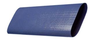
The Model PD1 is a blue PVC discharge lay-flat hose that resists kinking and twisting. It is designed as a standard duty hose for water discharge in industrial and construction applications, is strong and economical, and rolls up flat for easy storage. Reinforcement includes spiral plies and longitudinal synthetic cords for excellent burst resistance. Other varieties for higher pressures alternate materials are also available.
