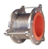
The Model Sanitary NLC metal bellows expansion joints utilize an integral silicone liner for food and similar service requiring a smooth bore. This Clean in Place (CIP) design (up to 8" diamters) greatly helps to simplify piping system design in systems that require service without convolutions that can trap solid media.
