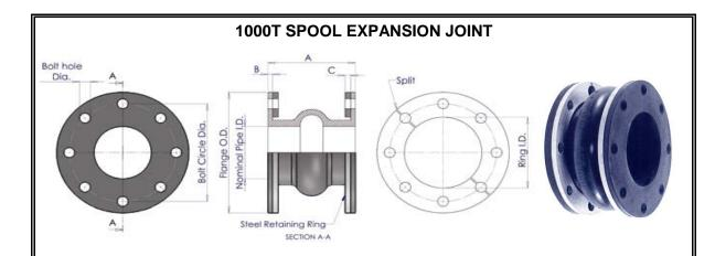
The 1000T Spool expansion joint is a molded arched spool rubber expansion joint for moderate pressures and movements. They are available in butyl and EPDM. Higher pressures and movements are available in the Ultraspool rubber expansion joint, and with PTFE lined as the Tefspool expansion joint
