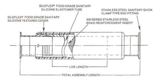
Available with clamp type, bevel seat and nut, cam lock, flanged or threaded in T304 or T316 stainless steel.
